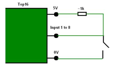
Inputs must be pulled high or low by connecting to 5V or 0V with a 1k to 10 k resistor. The diagram above shows the input normally high (logic 1), closing the switch will bring the input low (logic 0).
