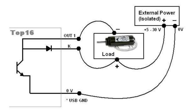
0V is also USB ground, Ground-loops can occur between the external supply negative and the Top16 0V. To prevent this, the external supply must be isolated from ground (transformer supply), or share a common ground with the PC.
